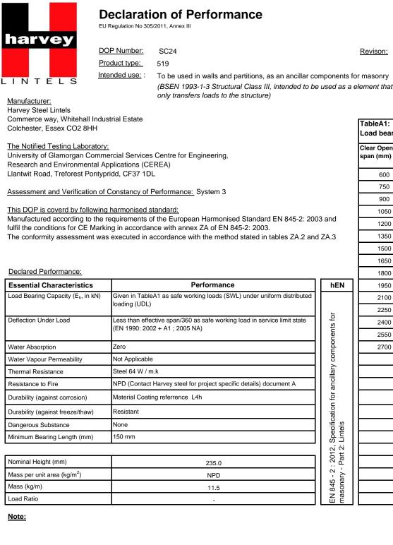
TableA1: Load bearing capacity Clear Opening SWL UDL (kN) span (mm) 600 28 750 28 900 21.4 1050 16.4 1200 13 1350 10.5 1500 8.7 1650 7.3 1800 6.2 1950 5.4 2100 4.7 2250 4.1 2400 3.6 2550 32 2700 2.9
